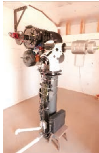
M.J.'s setup: New astrophysics mount, with CDK 14 scope on top and 11" Celestron scope on bottom
